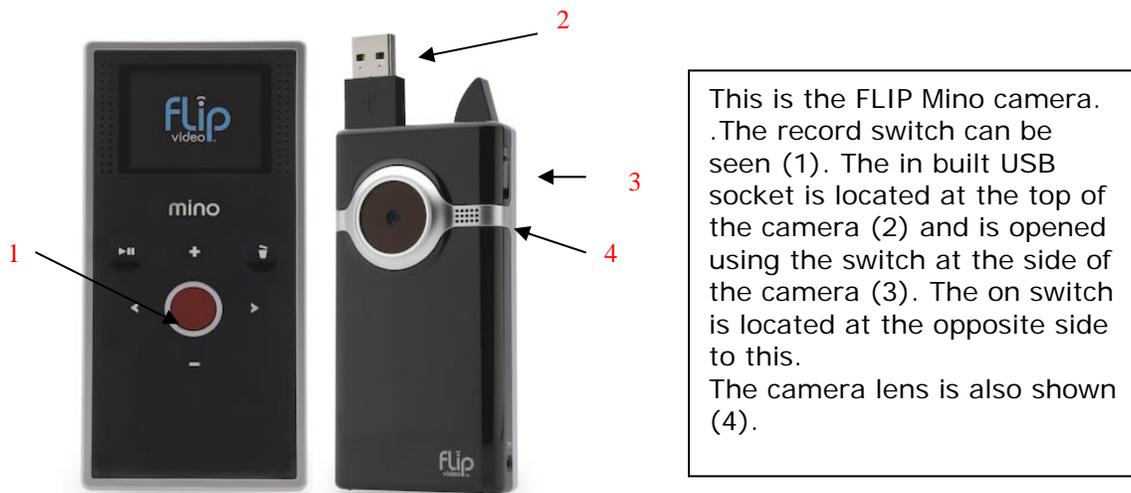
**Figure 3.** The FLIP Mino Device
